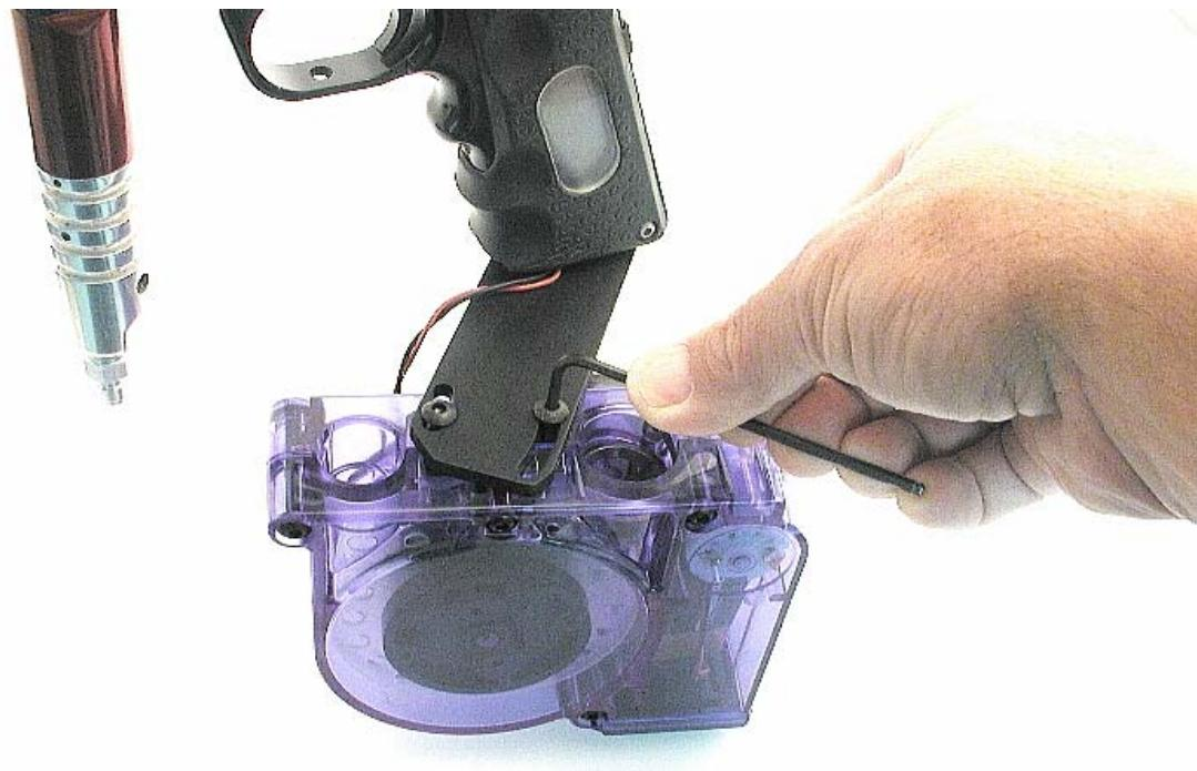
**The slotted end of the mounting bracket allows you to adjust the position of the Warp.**
