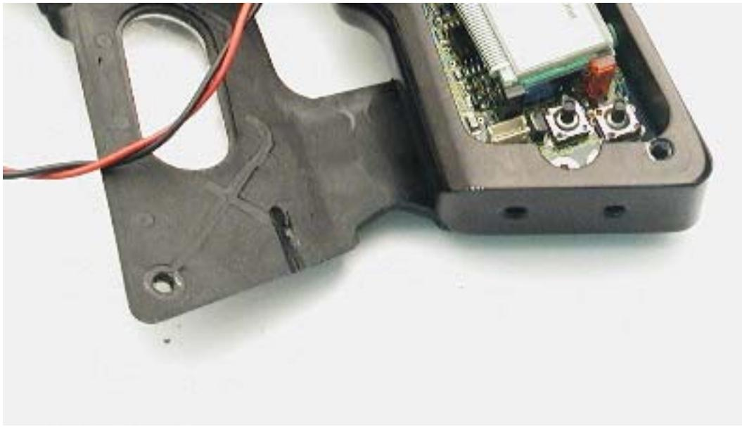
**Test fit the harness wires and adjust the cut as necessary. The notch should be a bit smaller than the width of the harness wires to help prevent it from being pulled out.**
