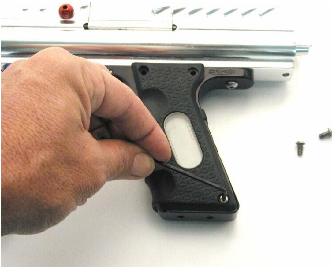
**Remove the three screws from the LCD side of the grip.**
