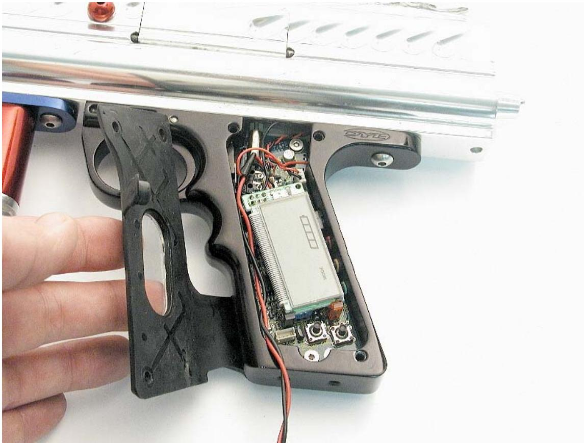
**Run the harness down and towards the front of the grip as shown. Close up the grip while aligning the wire with the notch you made.**
