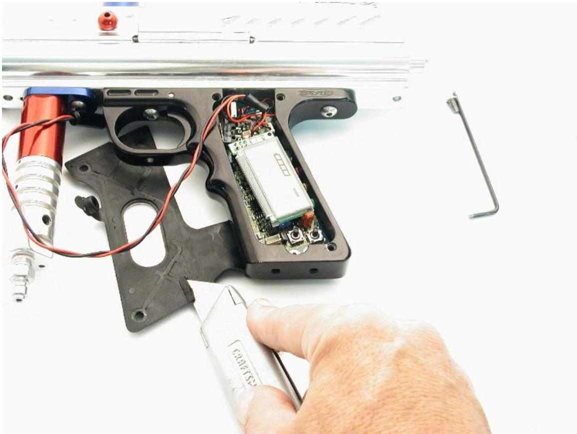
**With the utility knife, carefully make a small “V” shaped notch  $\frac{1}{2}$  inch long on the inside of the grip as shown. Be careful not to cut all the way through!**
