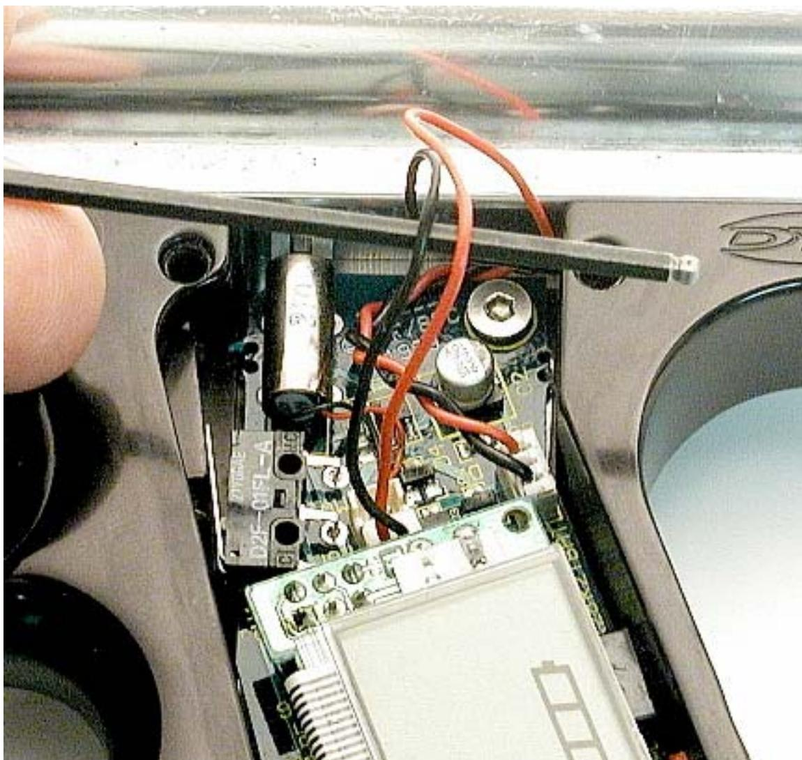
**Note that the wires are plugged into a double socket and the side nearest the display.**
